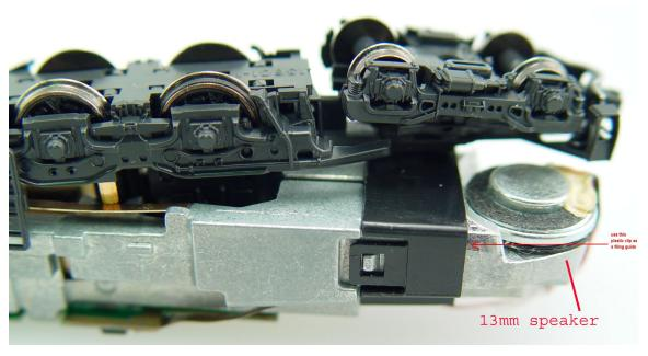
Using the larger 13mm round speaker increases the volume. After this modification, you should be able to hear the loco from 10 feet away or more.
