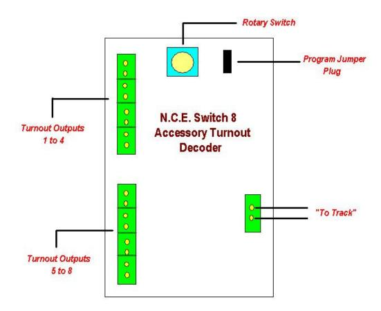
To program each other Switch 8 you have to re program each output individually, there is no master address to set all 8 outputs simultaneously.
