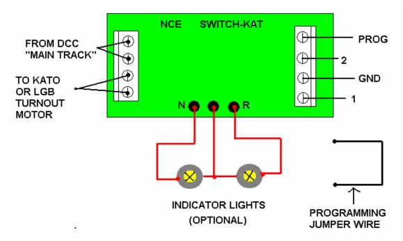
Once done with wiring the Switch-Kat properly, go to page 4 of the NCE instruction booklet for "Programming Information" to make sure you have the "Programming Jumper Wire" attached to the "PROG" and "GND" terminals of the Switch-Kat, (see above diagram).
